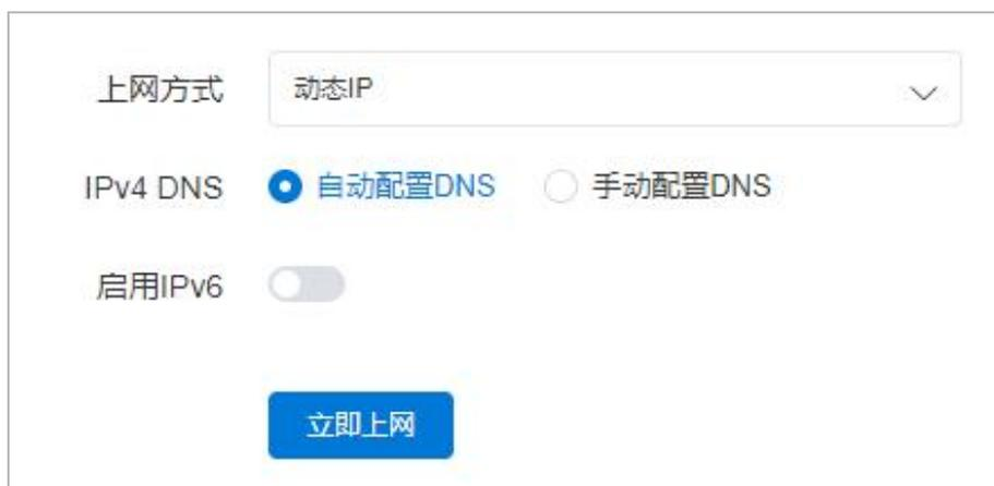
The screenshot shows a configuration form for dynamic IP. The '上网方式' (Internet Method) dropdown is set to '动态IP' (Dynamic IP). The 'IPv4 DNS' section has radio buttons for '自动配置DNS' (Selected) and '手动配置DNS' (Manual). The '启用IPv6' (Enable IPv6) toggle is turned off. A blue '立即上网' (Connect Now) button is at the bottom.
